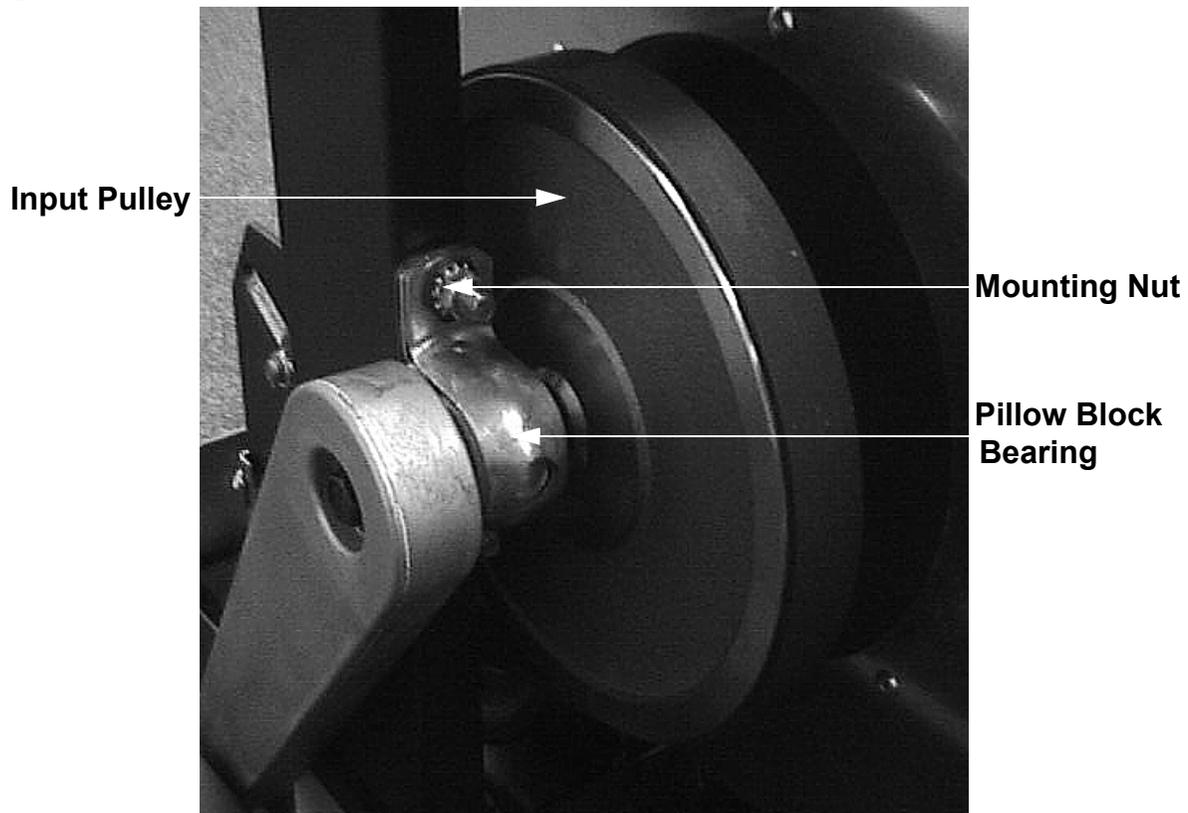
**Diagram 7.10 - Pillow Block Bearings (serial code AA23)**
