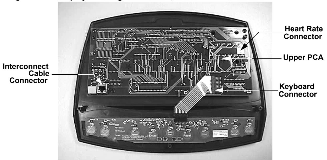
7. Position the replacement upper PCA at its mounting location on the display housing front panel (refer to Diagram 7.3). Replace and tighten the upper PCA mounting screws.
