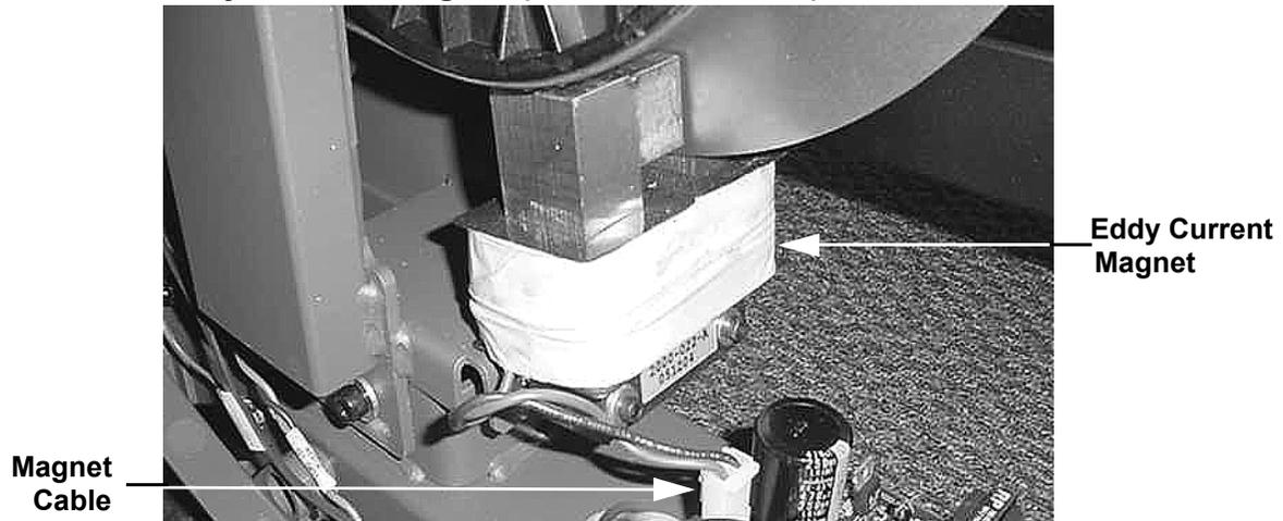
4. If the resistance measures significantly less than  $90 \Omega$  or significantly more than  $110 \Omega$ .
