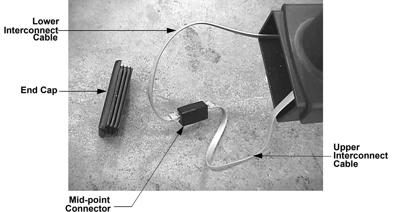
4. If you are replacing the upper interconnect cable skip to step 9. If you are replacing the lower interconnect cable continue with step 5.
