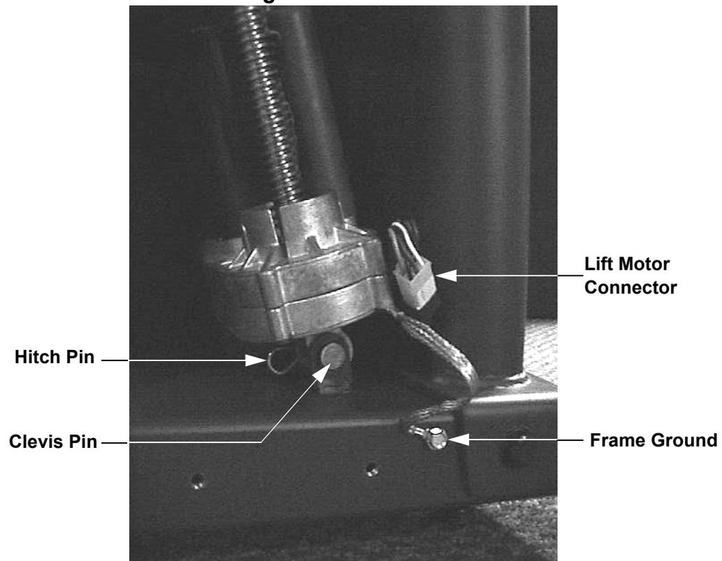
9. Depending on the manufacture date of the 5.23, the lower end of the lift motor will either be fastened with a clevis pin and hitch pin or with a bolt and nut. Unfasten the lower end of the lift motor and remove the lift motor from the unit.
