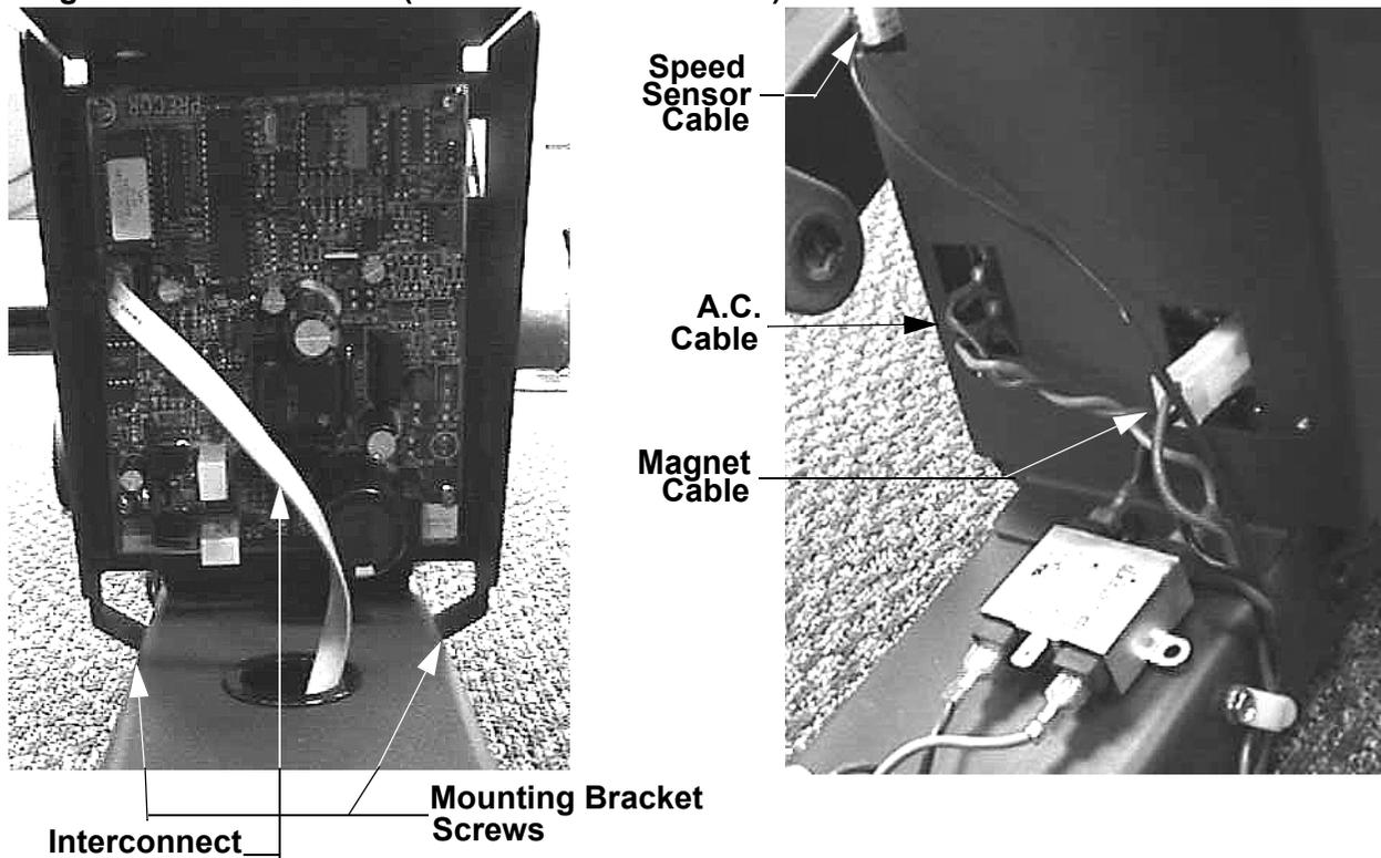
6. Carefully, rotate the lower PCA mounting bracket away from the front cover section and disconnect the interconnect cable from the lower PCA. Remove the lower PCA and mounting bracket from the unit.
